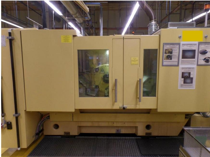
The KRONOS S 250 is designed for workpieces in the diameter range of 1.5 to 35 mm. It offers plunge cut and throughfeed grinding method with a plunge cut width up to 245 mm. It is the perfect machine for mass production of small precision workpieces.
