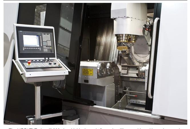
The LIECHTI Turbomill 800g is a highly dynamic five-axis milling machine with maximum axis acceleration, designed for high-speed milling in 5 axes.
