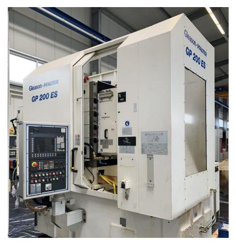
CNC gear shaping machine for shaping internal and external spur and helical gears. Due to the electronic helical guidance also very well suitable for small lot sizes and prototypes.
