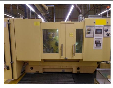
The KRONOS S 250 is designed for workpieces in the diameter range of 1.5 to 35 mm. It offers plunge cut and throughfeed grinding method with a plunge cut width up to 245 mm. It is the perfect machine for mass production of small precision workpieces.
